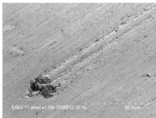
Fig.7 SEM micrograph of the corrosion pit
