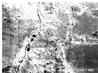
Fig.6 SEM photograph of the specimen surface ( S=30\text{MPa} )
