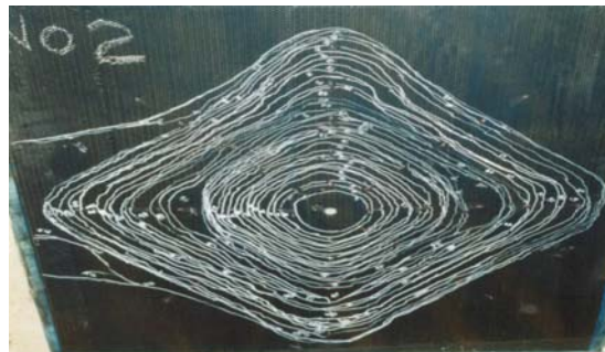
Photo.1 Progress of peeling off zone (No. 2)
