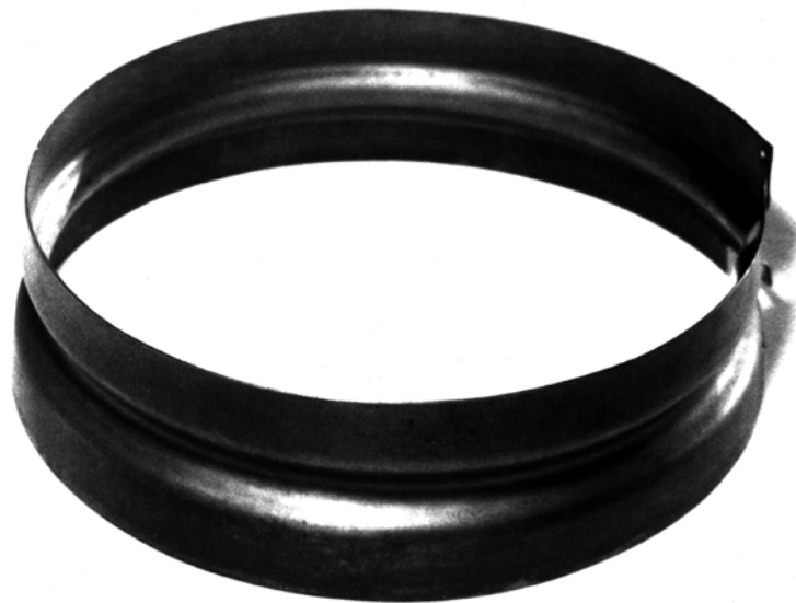
Fig.5: An item manufactured by explosive stamping from a low-ductility titanium-base alloy coated with a plasticizing film
