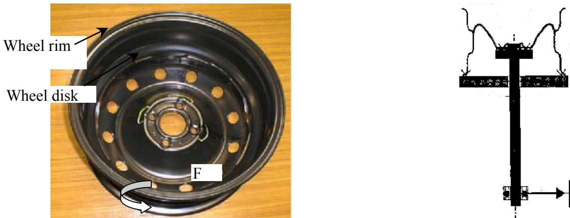
Figure 3: FB600 wheel and outline of the fatigue method
