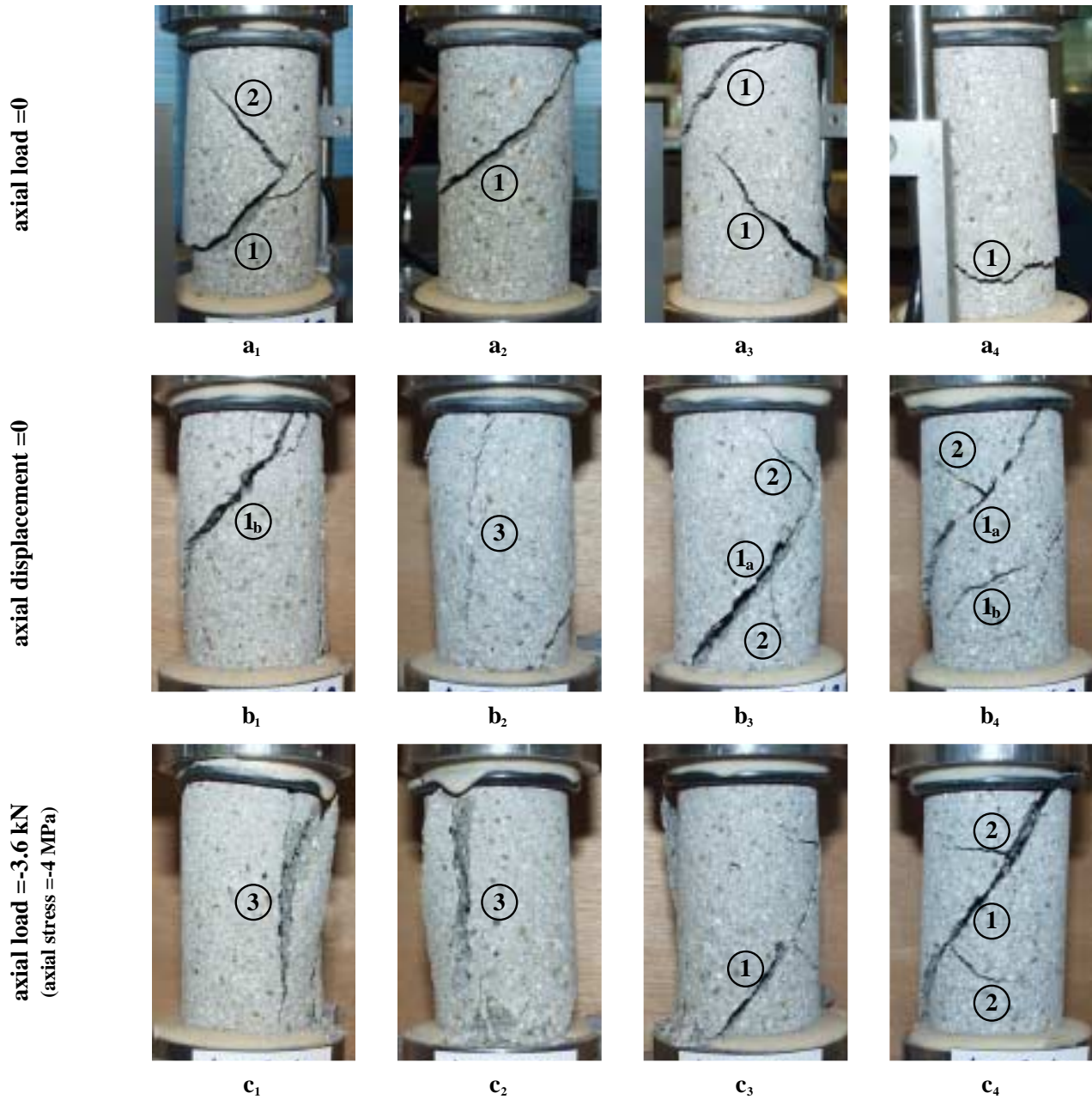
Figure 2: Experimental results obtained with un-notched specimens under zero axial force (a), zero axial displacement (b) and constant compressive load (c)
