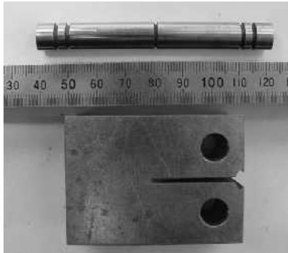
Figure 2 A valid ASTM CTT specimen (bottom) compared to cylindrical CNT specimen for the same material.
