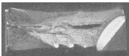
Fig.1 Macro-profile of the fracture surface of a SECC specimen
