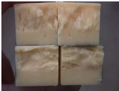
Figure 3: fractured surfaces showing directional properties
