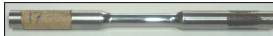
Figure 3. Photo of a rotating bending fatigue test specimen which attained fatigue life over 10^6 cycles.
