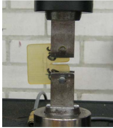
Figure 2. Quasi-static testing of CT specimen with the loading fixture
