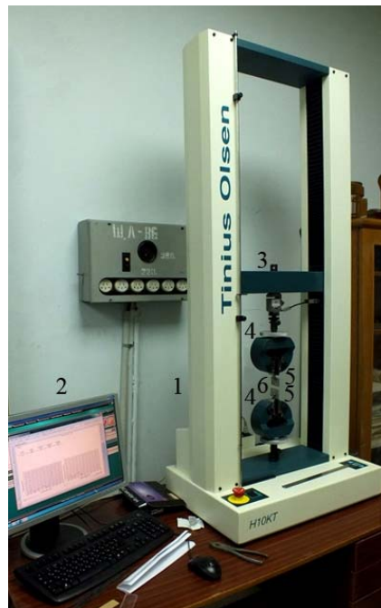
Fig. 1. General view of the test machine: 1 - frame, 2 - PC 3 - moving cross-arm, 4 – machine's grabs, 5 - sample clips, 6 – sample.
