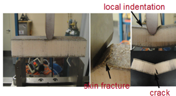
Figure 4. Three-point bending experiment set-up and main failure modes
