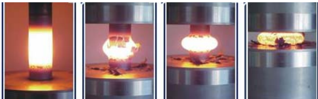
Figure 1: Integrated thermo-mechanical forming process of the flange shaft [6]
