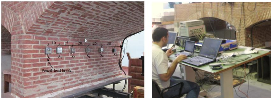
Figure 2. Wave velocity test: (Left) the sketch of the pencil-lead break point and the sensor distribution; (Right) scenario of the velocity test.
