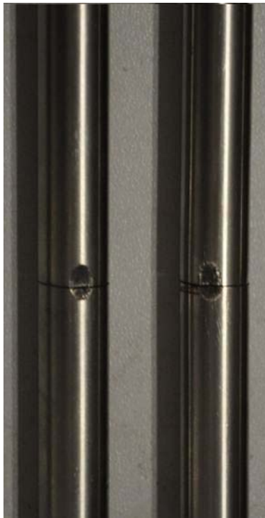
Figure 4. Fretting scars and cracks of specimen no.9 and no.10
