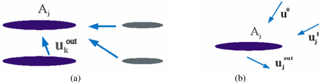
Figure 2 Illustration of pseudo-incident waves (a) scattering from other defects, (b) total incident wave for a defect
