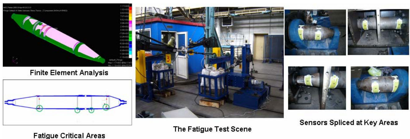
Figure 6 Some works done for extending the fatigue life of the shaft in a type of fighter aircraft
