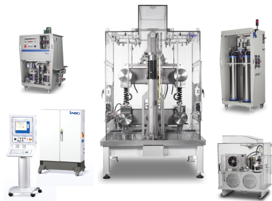
Figure 9. Corrosion Spring Testing Machine [IABG]
