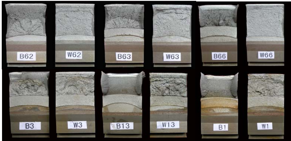
Fig.6. fracture cross-section of different CTOD specimens
