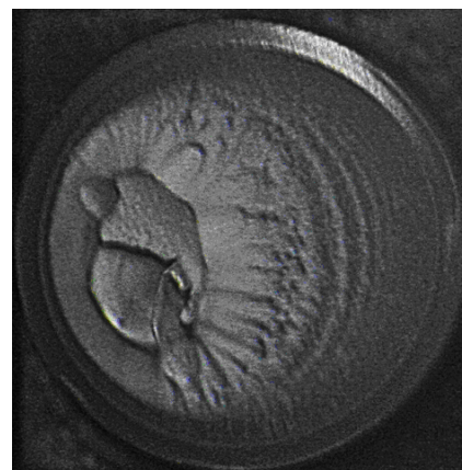
(b) Asymmetric fatigue crack growth
