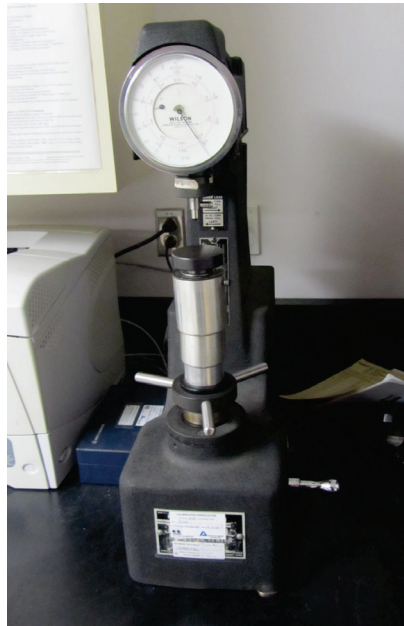
Figure 2. Wilson Rockwell 3TT Twin Hardness Tester
