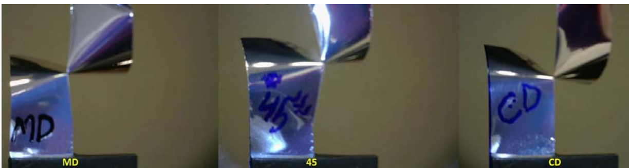
c ) final trouser tearing, edge effects may come into consideration
