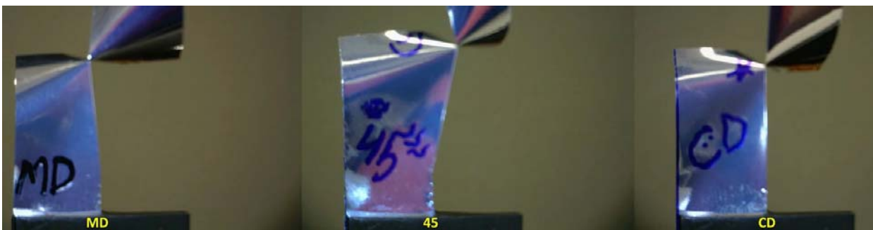
d ) finalized trouser tear test
