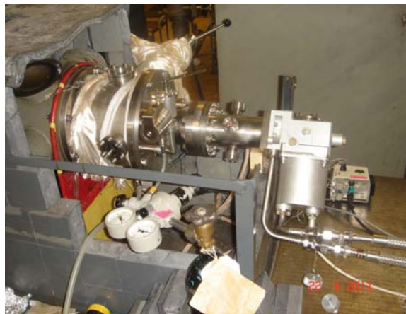
Fig. 2. Appearance of the research camera and gases inlet system .
