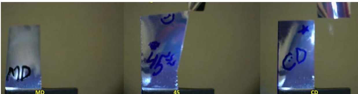
d ) finalized trouser tear test
