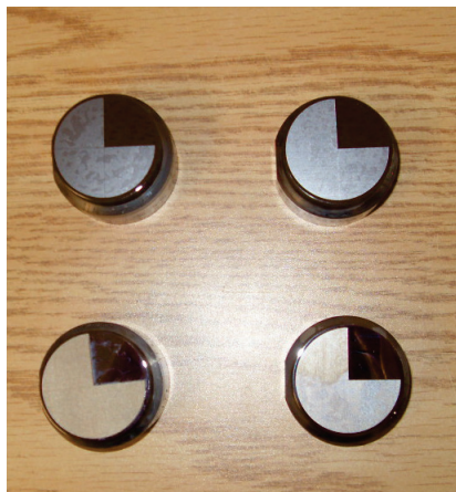
Figure 3 Test dies with three-quarter laser frosted surfaces
