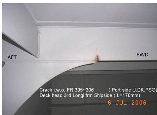
Figure 2. A fatigue crack in the case study vessel and the structural detail in the fracture analysis.
